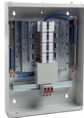
8 Way TP&N MCB Board c/w 100A TP Incomer
